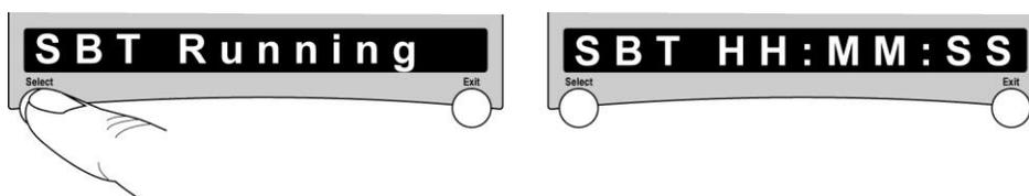
When an SBT procedure is active, **SBT Pres. Sup**, **SBT PEEP** and **SBT O<sub>2</sub>** monitored values are displayed in the front panel **Pres. Support**, **PEEP** and **O<sub>2</sub>** control display windows, respectively.
