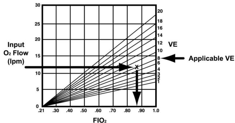
Example - To determine the delivered O<sub>2</sub> concentration
