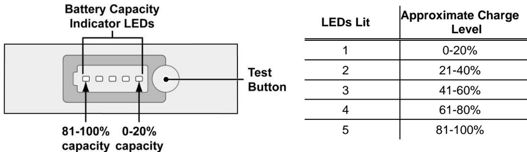
If the battery is being charged, the LED that is representative of the of the battery’s current charge level flashes while the test button is being pushed.
