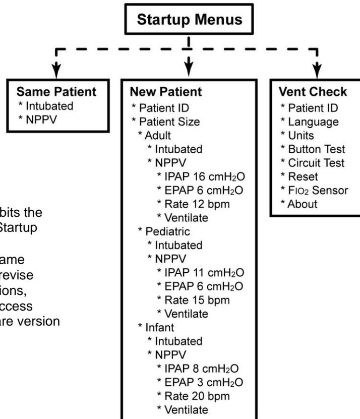
While in Startup mode, the ventilator inhibits the normal delivery of gas and displays the Startup menus.
