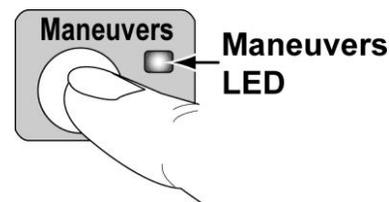
Maneuver arming automatically terminates if 60 seconds elapse in the same phase of a maneuver without a button press.
