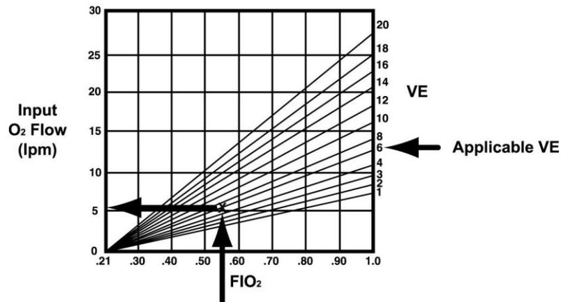
Example - To determine the required O<sub>2</sub> input flow
