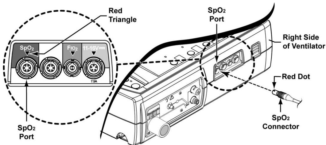
triangle) and will lock into place when properly inserted
