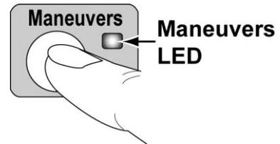
The maneuver will occur while the **Maneuvers** button is held for a maximum of six (6) seconds. If the button is released before the six seconds has expired, the maneuver will be terminated. In either case, the ventilator returns to normal ventilation immediately following termination of the maneuver.
