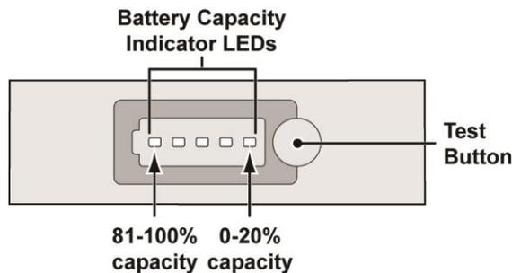
If the battery is being charged, the LED that is representative of the of the battery's current charge level flashes while the test button is being pushed.
