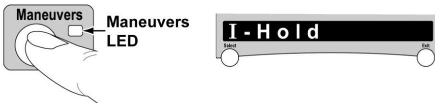
To perform an Inspiratory Hold, arm and run the maneuver as follows, or to perform an Expiratory Hold, rotate the **Scroll** knob until **E-Hold** appears in the display window, then proceed as follows.
