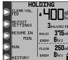
Figure 18B. HOLDING mode options, intermittent feeding mode.
