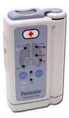
The Panorama Telepack-608 is a battery powered ambulatory device that acquires ECG information from an adult patient and transmits it to the Panorama Telemetry Server for data analysis functions such as heart rate determination, R-wave detection, ECG filtering, and arrhythmia recognition.
