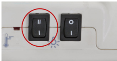
Figure 3-8 : Irradiance selection switch
