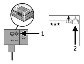
3. Charge the system for 4–5 hours or until the battery gauge icon indicates a full charge.
