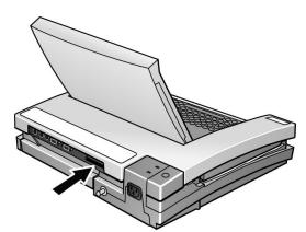
To remove the SD card from the slot, press the card into the slot; the slot is spring-loaded and will eject the SD card.
