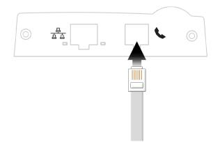
To connect to the external modem, you must first install the external modem kit. See the Field Service Manual for instructions on mounting and connecting the external modem kit.
