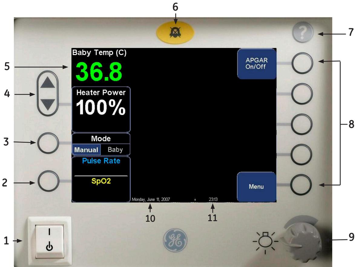
Figure 5: Control panel and color screen display
