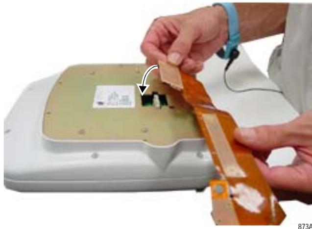
5. Using two screws, secure the flex cable to the display assembly.
