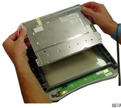
3. Dampen a clean, soft cloth with window cleaner and carefully clean and dry the LCD display and the display filter to remove fingerprints and dust particles.
