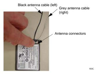
m. Insert the wireless card (with the antenna connectors facing down and the connected antenna cables on the righthand side) into the PC card bracket.
