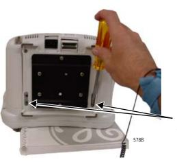
Note: Use a screwdriver with a long blade or remove the GCX plate first for easy access to the bottom screws.
