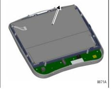
Use a 5 mm nut driver to remove the four stand-off screws anchoring the display to the rubber display isolator.
