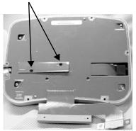
Flip over the display shield flex circuit. Disconnect the display shield cable from the backlight inverter PCB.
