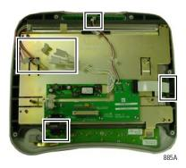
Remove the four screws anchoring the mounting plate to the LCD display.
