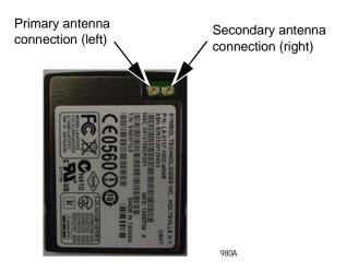
The relationship between the wireless card connectors, wireless antenna cable colors and the primary/secondary antenna signal strength test settings are as follows:
