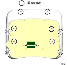
3. Separate the transition bezel from the front bezel. It is not necessary to remove the metal backplate.
