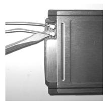
6. Reconnect the antennas connectors to the replacement wireless card. The black antenna cable connects to the connector on the left and the grey antenna cable on the right.
