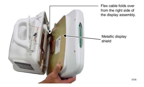
5. To prevent damaging the display flex cable, position the display assembly for the patient monitor you are servicing.
