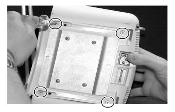
9. Carefully pull the CPU/battery housing assembly from the unit.
