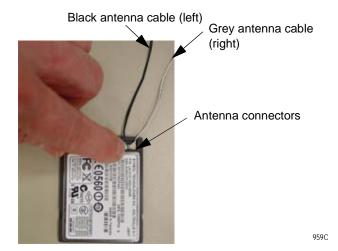
7. Reinsert the wireless card into the PC card bracket.
