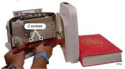
9. Carefully align and insert the DAS cable pins into the DAS assembly until the snap latch clicks into place.
