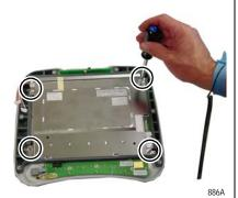
e. Lift out the LCD display from the rubber display isolator and set aside.
