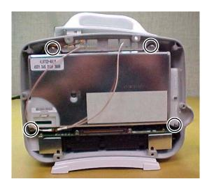
4. Remove the DAS assembly by first pulling the *left* side out 1/4-inch, then sliding the whole assembly out of the patient monitor. If the Wireless LAN option is installed, use a needle nose pliers to remove the antennae by disconnecting both coax connectors from the compact flash card.
