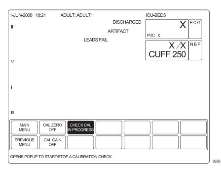
8. Select *CHECK CAL IN PROGRESS > STOP*. The patient monitor automatically releases pneumatic pressure in the entire plumbing circuit.
