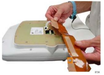
5. Using two screws, secure the flex cable to the display assembly.
