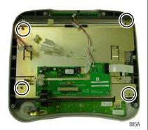
c. Remove the mounting plate and set aside.
