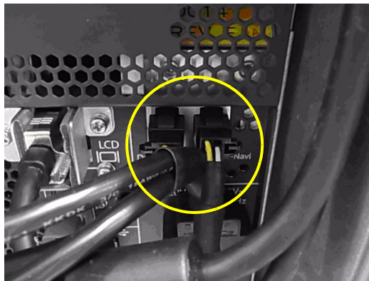
Figure 8-103 Remove VNAV Option power cable connector from system
