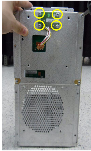
Figure 8-66 Removing the CSI Assy
