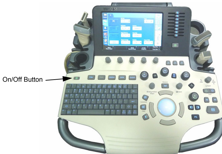
Figure 3-11 On/Off Button on Control Panel
