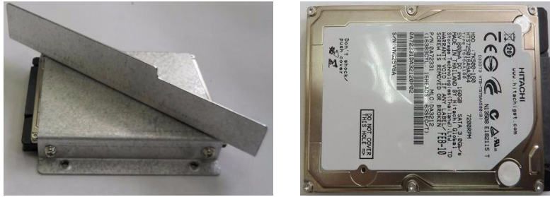
Figure 8-74 Removing the hard disk bracket
