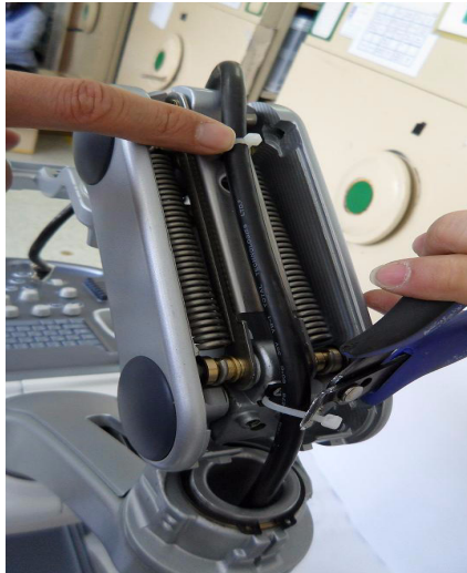
Figure 8-131 Removing the cable ties
