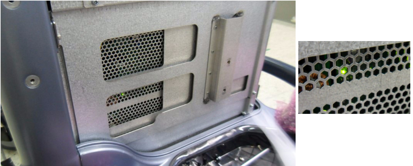
Figure 7-1 check green LED inside CPS
