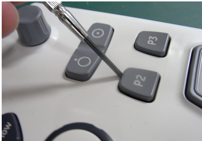
Figure 8-39 Push against the circle cap and lift it
