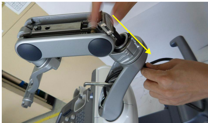
Figure 8-133 Pulling out Harness cable
