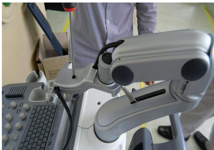
Figure 8-129 Removing the 3rd arm cover
