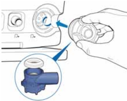
Figure 2-3 Installing the expiratory valve
