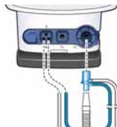
Figure 5-7 Connecting the flow sensor to expiratory valve, nCPAP-PS mode
