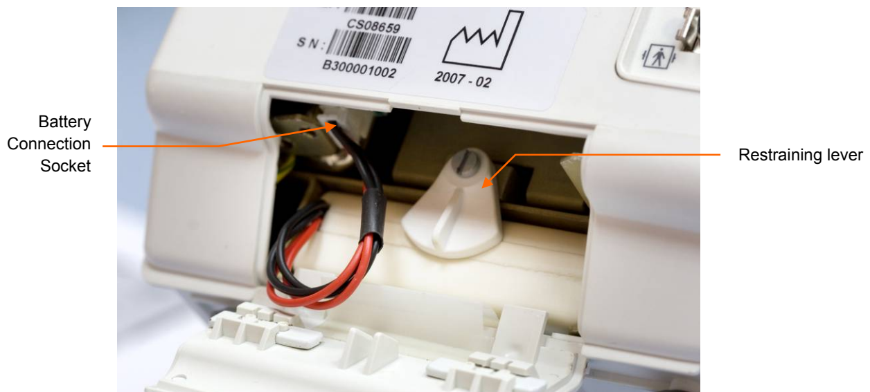
Figure 2 - Battery Pack Close-up
