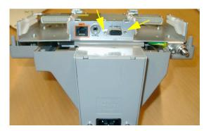
5 Remove the two screws on the main board.
