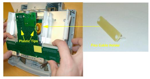
7 Unplug the flex cable from the main board and remove the board.
