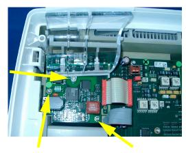
3 Lift the board out to the right so the ECG out connector is pulled out of the monitor housing.
