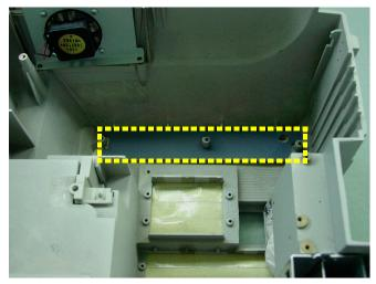
**CAUTION** Make sure that none of the circled parts shown below are bent or damaged in any way. If they are damaged, return the power supply.
