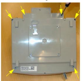
Remove the four screws securing the metal plate and lift it off.
