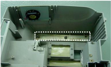
2 Remove the protective layer from the new heat conducting foil, place the foil over the domes and press it onto the power supply assembly using your thumbs.
