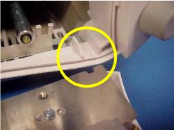
3 Unscrew the screws holding the flex panel adapter cable and pull off the flex cable carefully towards you.
