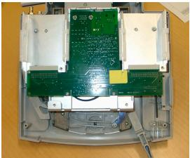
4 Remove the two screws next to the video connector.
