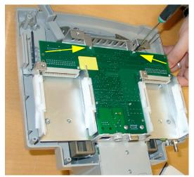
6 Push the platic tips through the board, lift the board up and remove the flex cable holder under the board.
