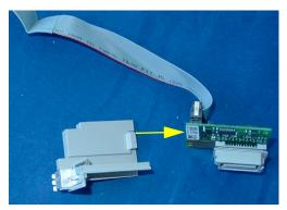
Reassembly Note: The MSL board and its housing must be properly aligned. Push down on the spring to slide the board into its position.
