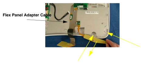
3 Pull out the silicon mat (for power switch and LEDs).
