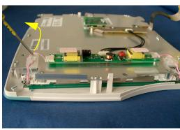
**Reassembly Note:** Cables must be re-inserted into the plastic cable holder with a slight strain on them towards the backlight tube. The cable holder functions as a strain relief.
