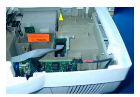
4 Pull the MSL board out of its housing if required.
