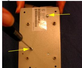
2 Remove the two remaining screws from the bottom cover of the IIT box.
