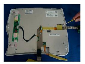
7 Unscrew the three screws and remove the flex panel adapter cable.
