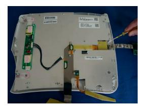
7 Remove the eight screws and carefully lift off the display assembly by releasing the two snaps in the monitor bezel.
