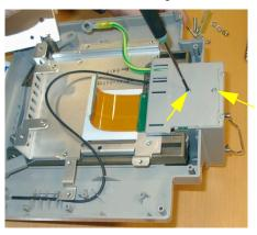
**Reassembly Note:** When reassembling the bottom cover of the power block, make sure that the grounding cable, the optic fiber and the flex cable run through the holes provided in the cover.
