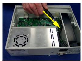
4 Lift the fan out of the battery conditioner housing.
