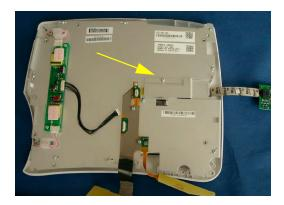
6 Slip a screwdriver under the end of the flex panel adapter cable and lift upwards to remove the connector to the display.
