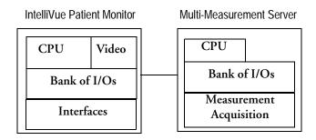
The CPUs provide two LAN interfaces to interconnect CPUs (via the MSL) and to connect to the Philips Clinical Network.
