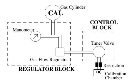
Figure 32 Block diagram - Internal Components
