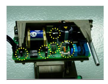
3 Insert the Power Supply into the monitor rear housing as shown below. Make sure the power supply snaps into the domes and is properly aligned with the screw holes.
