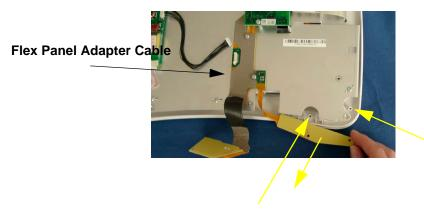
4 Remove the eight screws and carefully lift off the display assembly by releasing the two snaps in the monitor bezel.
