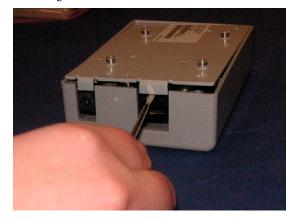
3 Turn the IIT box around and lift the top cover off completely. Then unplug the flex cable from the PCA board.
