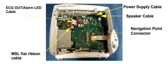
**NOTE** To remove the flat ribbon cables with red connectors (e.g. Navigation Point cable) simply pull directly on the cable. The MSL, power supply and speaker cables have different security locks and must be unlocked in order to be removed.
