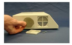
3 Re-insert the mat and refit the cover and screws.
