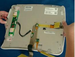
**CAUTION** We recommend that this procedure is performed in a dust free environment. The display assembly may be hard to remove from the touch panel due to the gasket (adhesive strips) holding the two together.
