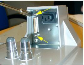
4 Remove the two screws from the bottom cover of the power block.
