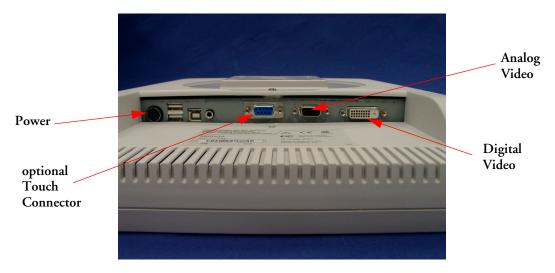
Figure 24 Connections M8033A
