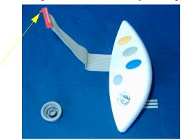
**Reassembly Note:** When re-inserting the input device, make sure the spring is inserted into the hole in the plastic housing.
