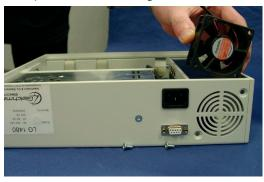
5 When replacing the fan make sure the connector is plugged in correctly as shown in the photograph below.
