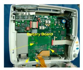
4 Unplug the Navigation Point connector, the MSL cable, the power suppy cable, the speaker cable and the ECG Out/Alarm LED cable from the main board.
