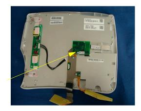
5 Unscrew the screw holding the metal sheet under touch controller board and remove the metal sheet.
