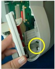
**NOTE** The screws securing the Navigation Point Assembly are self-cutting - turn in opposite direction first when re-inserting them.
