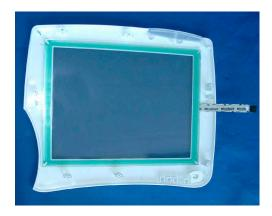
**NOTE** You must replace the touch panel and the touch controller board together in order for the monitor to function correctly.
