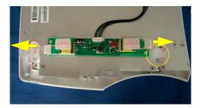
5 Unscrew the screw holding the metal sheet under touch controller board and remove the metal sheet.
