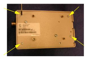
2 Lift up the bottom cover using a screwdriver.
