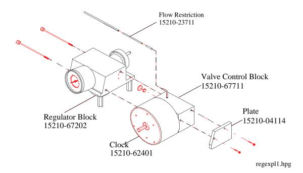
Figure 35 Exploded view - Regulator and Control Blocks
