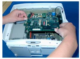
Reassembly Note: Hold the main board with your left hand on the plastic tip and re-insert it, making sure that the board is properly aligned with the protruding noses of the rear chassis and the slit for the internal module rack board and that the board is connected properly to the rack connector. The screws must be reinserted in the order specified in the picture above. Screw number 3 is attached to a black spacer which is not shown in this picture.
