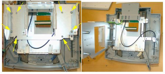
3 Remove the guide pins next to the flex connector on the front side of the power block.
