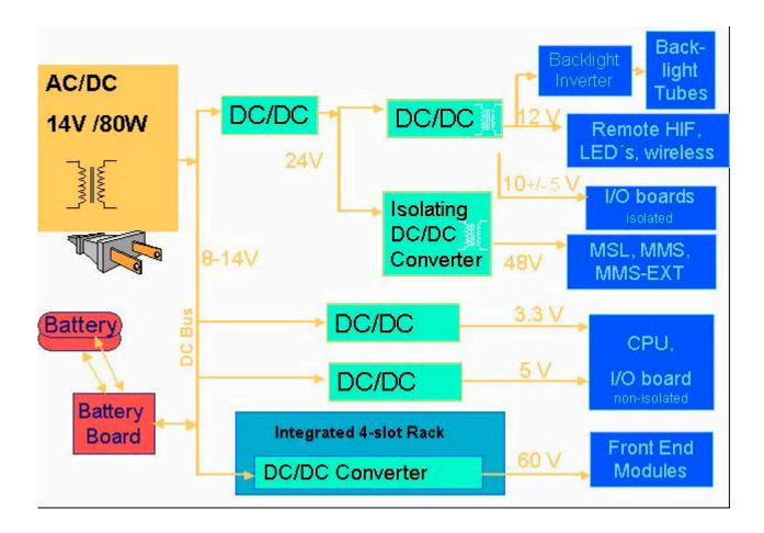
Figure 7 Power Supply Architecture
