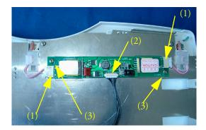
**NOTE** The backlight tube cable must not be unplugged for display exchange
