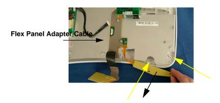
4 Remove one screw and then remove the touch controller board.
