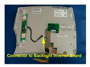
3 Remove the two screws securing the power switch and the LED board and pull out this part of the flex panel adapter cable.
