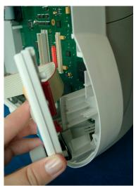
Reassembly Note: When reinserting the connector insert the protruding nose at the top
