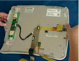
**NOTE** This procedure must be performed in a dust free environment. The display assembly may be hard to remove from the touch panel due to the gasket (adhesive strips) holding the two together.
