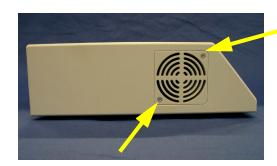
2 Remove the filter mat and clean the dust out by shaking.
