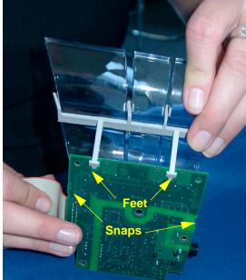
**Reassembly Note:** Make sure the snaps and feet are properly hooked into the ECG Out board when reattaching the lightpipe holder.
