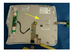
6 Slip a screwdriver under the end of the flex panel adapter cable and lift upwards to remove the connector to the display.
