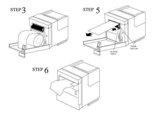
To load paper into the recorder module:
