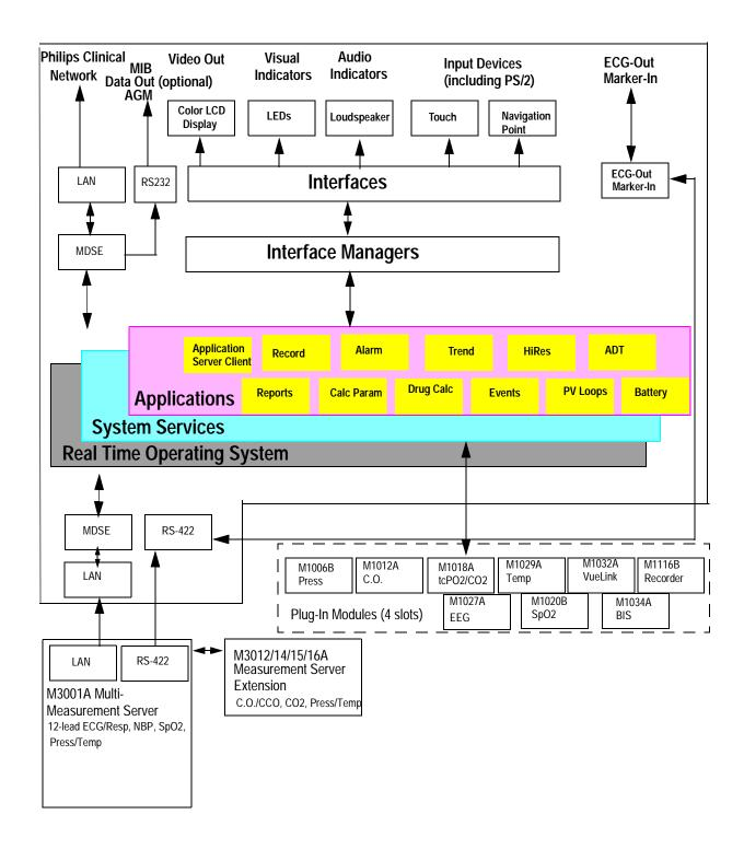
Figure 8 IntelliVue Patient Monitoring System Functional Block Diagram
