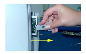
**Reassembly Note:** If you have installed #J35 (IntelliVue 802.11 Bedside Adapter) please attach the approval label or the WLAN label for Japan (country specific) and the antenna and connect the cable from the 802.11 Bedside Adapter to the wireless port as shown below.
