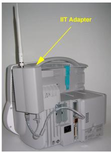
Figure 2 MP40/50 Rear with internal IntelliVue 802.11 Bedside Adapter (left) and with external IIT Adapter (US only) (right)
