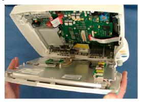
**Reassembly Note:** Make sure the metal sheet on the back of the display is inserted into the noses of the monitor rear housing when reassembling the two halves.
