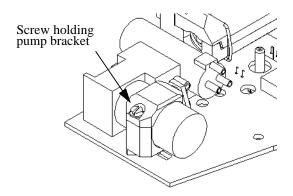
3 Gently disconnect the flow tubing attached to the Extension from the Pump.
