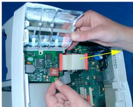
**NOTE** The connector must be unplugged from the main board.
