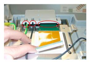
5 Remove the black Split Core and pull out the flex cable from the bottom.
