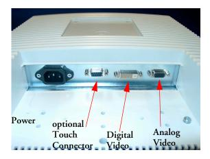
Figure 26 Connections M8033C
