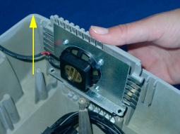
5 Remove the four screws to remove the speaker housing.
