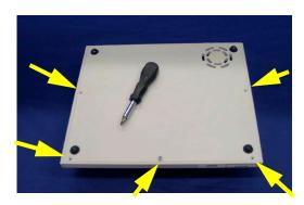
2 Lift the bottom cover up at the front and pull it off.
