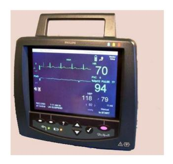
The M2636B TeleMon Monitor is a part of the M2601A Telemetry System -
