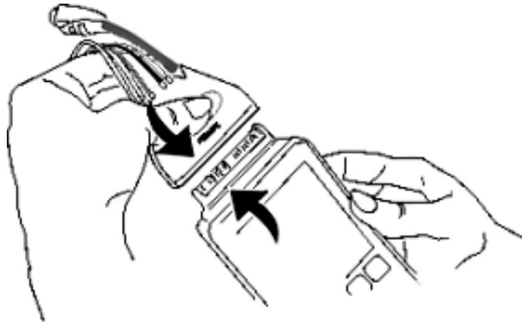
When connecting to the MX40, there is a slight clicking sound that signifies that the cable is securely connected.
