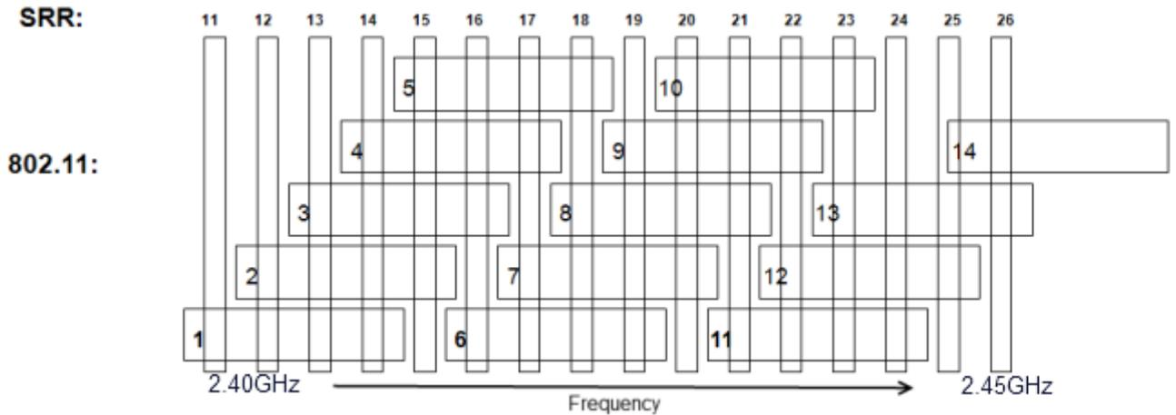
**Note** — Channel overlap as shown in this diagram is not totally accurate. There is not sufficient resolution to pick channels solely by using this diagram. Use it in conjunction with the tables provided.
