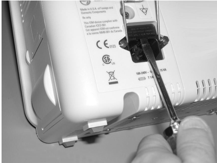
4. Replace the fuse(s), then push the fuse holder back into the power connector until it snaps into place.
