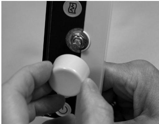
4. Remove the locking nut and washer.
