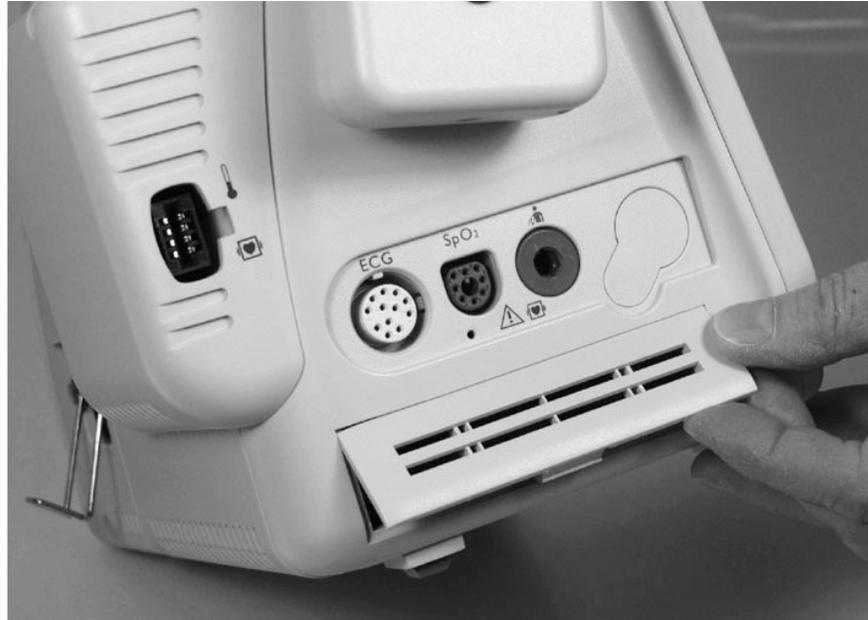
4. Snap the battery cover into place by pressing it firmly against the monitor case.
