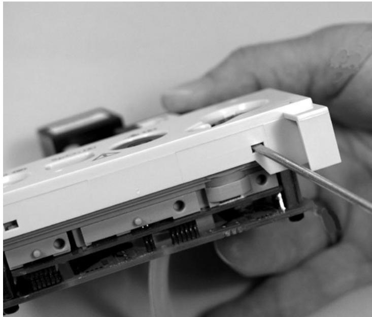
6. To reattach, line up the openings in the plastic cover with the patient connector tabs and snap the cover into place by pressing it onto the assembly.
