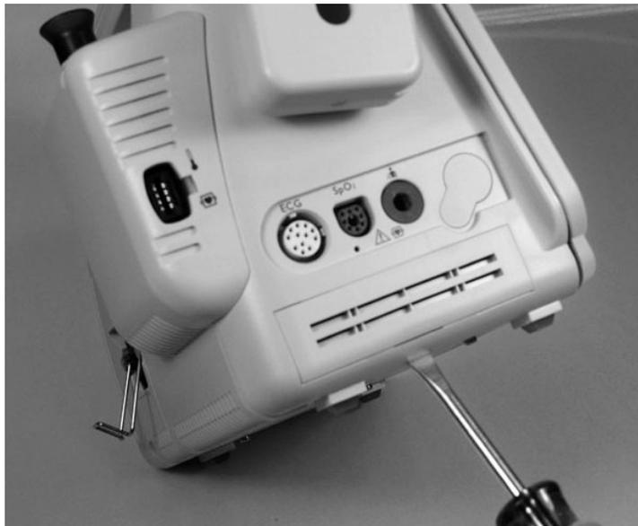
3. Slightly twist the screwdriver to pop the battery cover off of the case.
