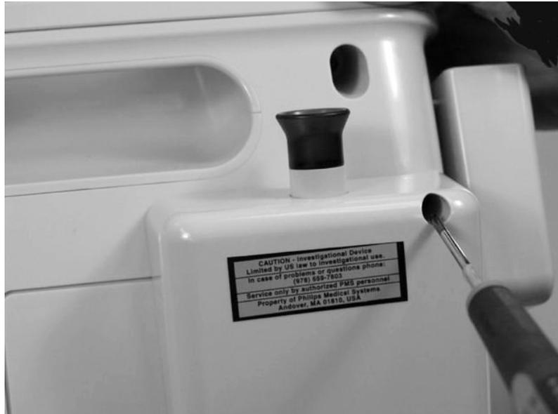
4. Remove three Torx T10 screws and washers from the bottom of the rear cover.
