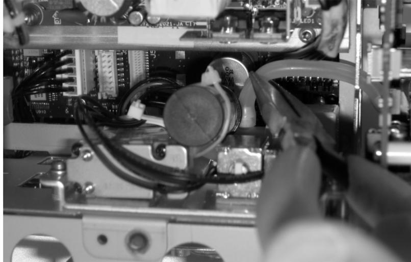
4. Remove the two Torx T10 screws and washers holding the front end assembly to the main PCB assembly metal case.
