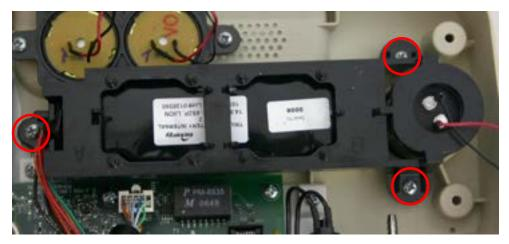
FIGURE 8-13: CAPACITOR/INTERNAL BATTERY FAN RETAINER SCREWS
