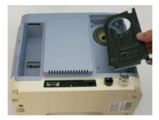
FIGURE 8-4: AIR PATH FOAM REMOVAL/INSTALLATION
