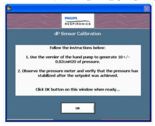
10. When the on-screen prompt below appears, press the relief on the hand pump to release existing pressure after connecting the hand pump tubing, then proceed with on-screen action (For Trilogy 200, Trilogy O<sub>2</sub>, & Trilogy 202 Only).
