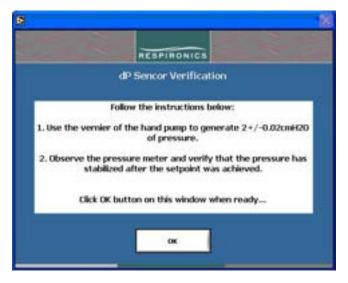
8. When the on-screen prompt below appears, press the relief on the hand pump to release existing pressure after connecting the hand pump tubing, then proceed with on-screen action (For Trilogy 200, Trilogy O<sub>2</sub>, & Trilogy 202 Only).
