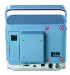
FIGURE 8-2: AIR PATH ASSEMBLY SCREW LOCATIONS
