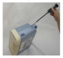
FIGURE 8-5: SCREW REMOVAL (REPEAT FOR OTHER SIDE)
