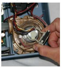
FIGURE 8-39: STIRRING FAN RETAINER REMOVAL
