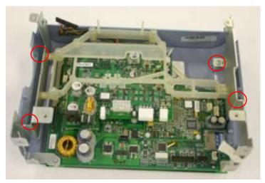
FIGURE 8-19: METAL BRACKET SUPPORT SCREW LOCATIONS
