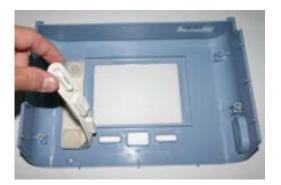
FIGURE 8-20: KEYPAD REMOVAL
