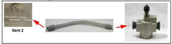
31. Connect one end of Smoothbore Tubing 18" to the other end of the Flow Control Valve. Connect the other end of the tubing to the inlet of TSI Model 4040 Flow Meter.
