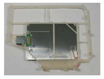
FIGURE 8-34: LCD CABLE REMOVED
