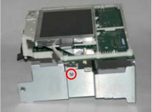
FIGURE 8-27: SCREWS SECURING THE METAL BRACKETS TO THE PCB SUPPORTS
