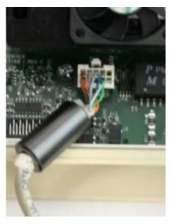
FIGURE 8-15: ETHERNET TO SYSTEM BOARD CABLE CONNECTION
