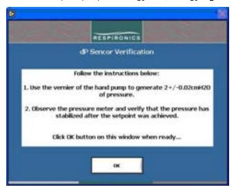
12. When the on-screen prompt below appears, press the relief on the hand pump to release existing pressure after connecting the hand pump tubing, then proceed with on-screen action (For Trilogy 200, Trilogy O<sub>2</sub>, & Trilogy 202 Only).
