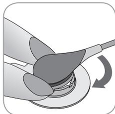
1. Hold the ring with one finger on every side of the sensor.
