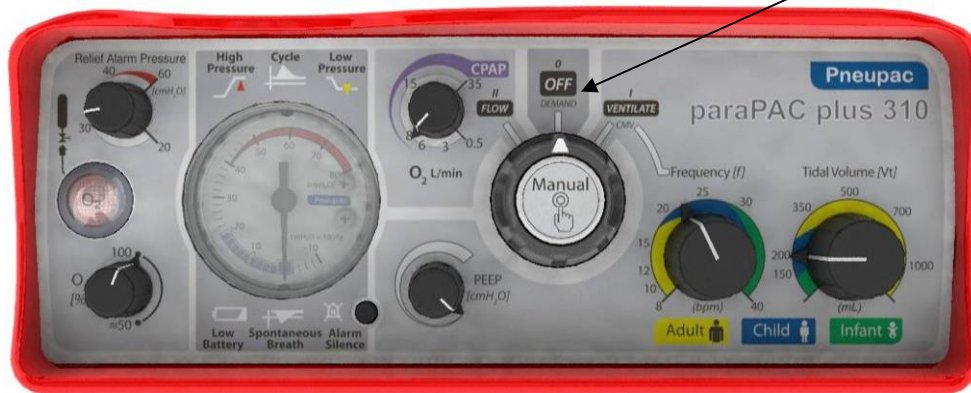
Figure 7: Selection for Manual Ventilation
