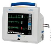
Extend telemetry surveillance outside your central antenna coverage area with the portable Ultraview telemetry monitor solution.
