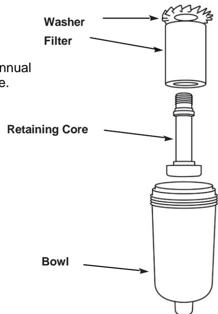
**Figure 4-1** filter assembly
