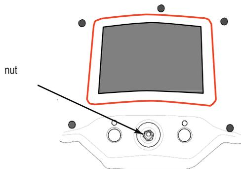
Figure 3-14 front panel with control knob removed
