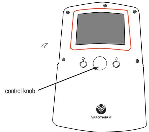
Figure 3-13 front panel with display cover removed
