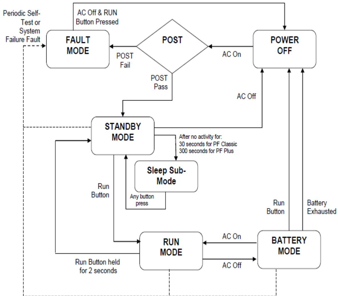
**Figure 1-3** Software Mode Diagram
