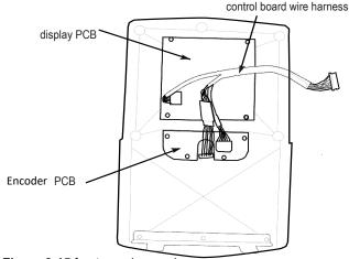
Figure 3-15 front panel- rear view
