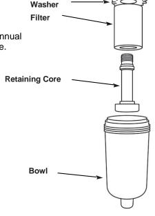
Figure 4-1 filter assembly
