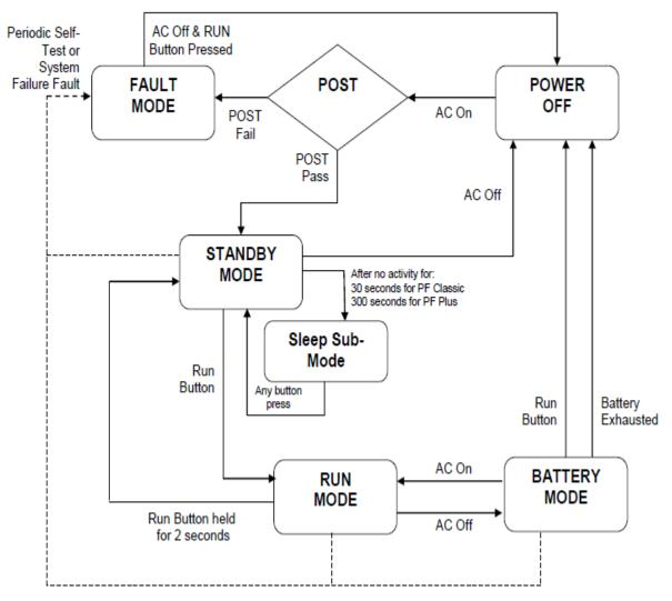
Figure 1-3 Software Mode Diagram
