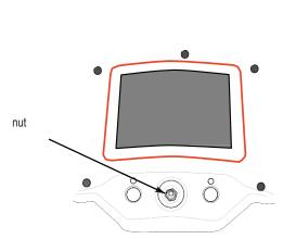
Figure 3-14 front panel with control knob removed
