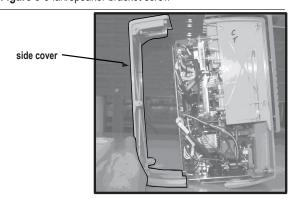
Figure 3-7 removing the side cover
