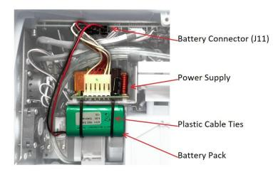
Figure 3-9 Power Supply/Battery Pack
