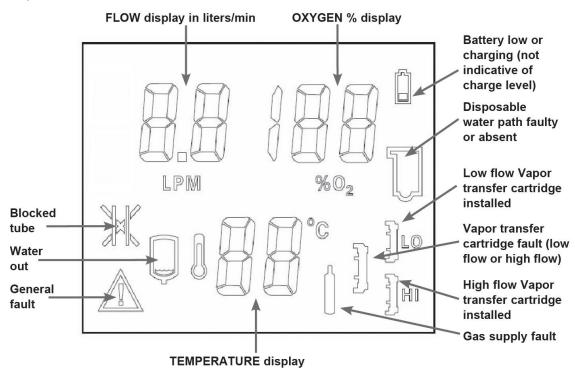
NOTE: LPM is noted as L/min on all newer Precision Flow devices
