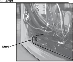
Figure 3-6 fan/speaker bracket screw
