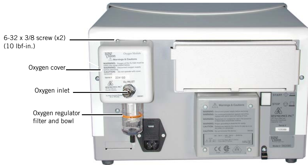
Figure 5-19: Removing the Oxygen Cover
