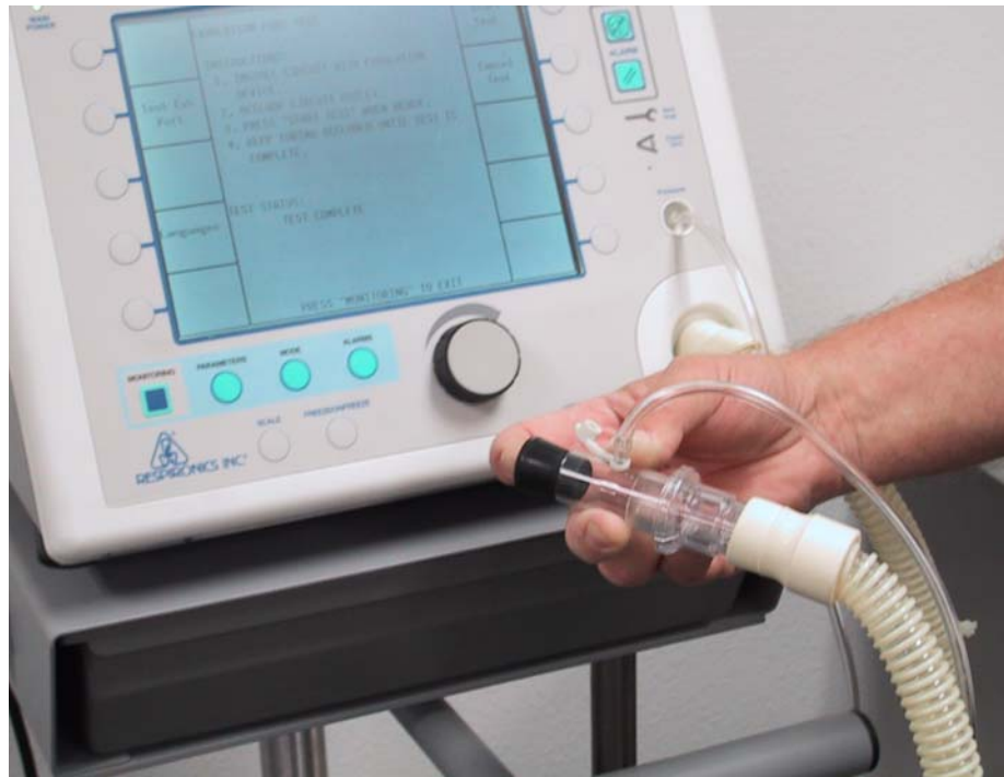
Figure 7-1: Exhalation Port Test Setup
