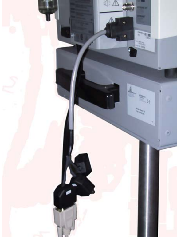
Figure 7-5: Setup for Transferring Total Hours for Newer or Upgraded Ventilator (s/n 106000 and above)
