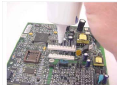
Figure 6-4: Applying Contact Grease to MC Board J1 Connector Pins
