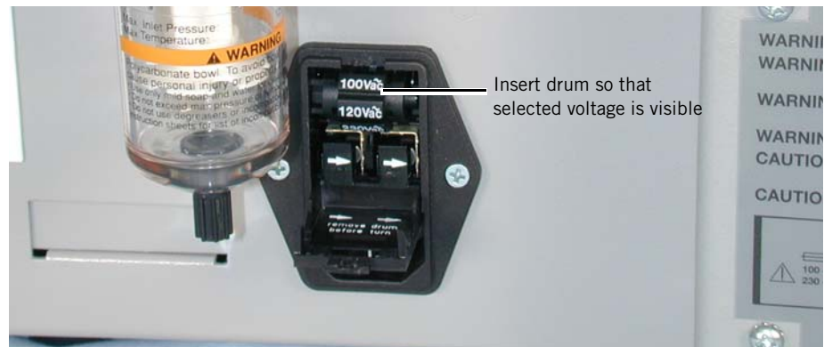
Figure 5-9: Selecting the Voltage
