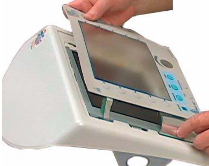
Figure 5-15: Feeding Touch Pad Cables Through the Front Panel
