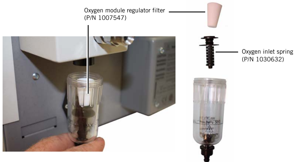
Figure 4-4: Removing the Oxygen Regulator Filter and Bowl (OM s/n 30000 and above)
