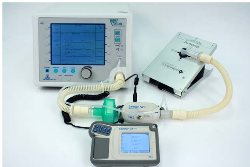
Figure 7-8: Dynamic Pressure Regulation Test Setup
