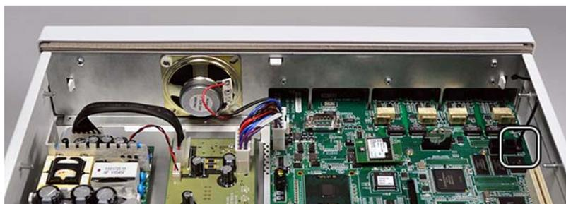
2. Remove 2 screws on front of bezel. Torque [1.1 Nm].
