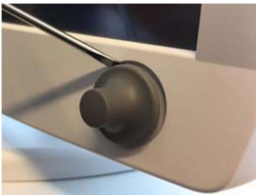
5. Use a screwdriver to disassemble the alarm light cover.
