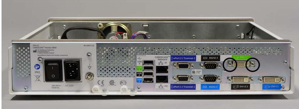
2. Remove 4 screws holding the video board. Torque [1.1 Nm].
