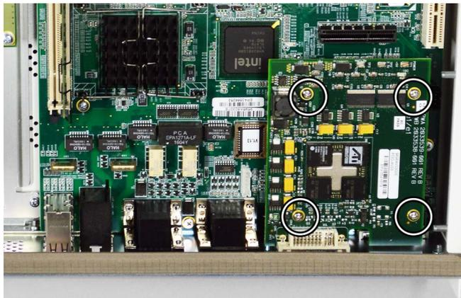
3. Lift the video card to disconnect the video card connector from the processor board.
