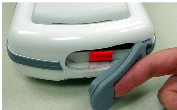
2. Pull the battery tray out of the PDM using the battery tray strap.
