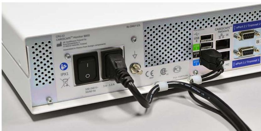
2. Secure the USB cables connections to the displays according to the instruction included in the display package.
