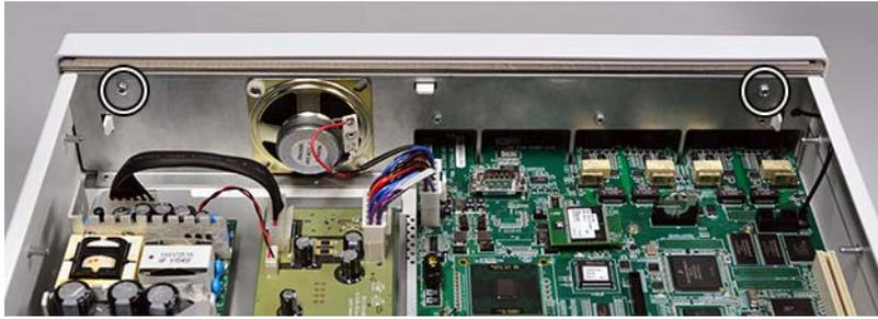
3. Release 3 snap fingers to free bezel from the front of chassis.
