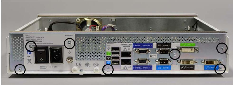
2. If the 3rd video card is installed, remove the 2 jack screws holding the DVI-I connector to the rear panel. Torque [0.6 Nm].
