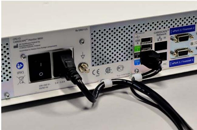
3. Disconnect all external cables connected to the CPU unit.
