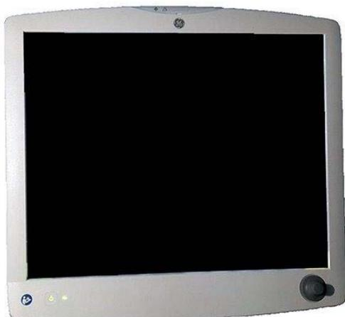
The display is a 19" touchscreen LCD with a Trim Knob control. The display provides both visual and audible alarms and connectivity to the USB input devices.
