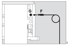
5 Insert the connector (F) of the flow sensor cable into the socket (G) at the rear of Evita V500.
