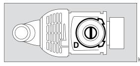
**4** Fit the diaphragm onto the edge of the fitting (D).
