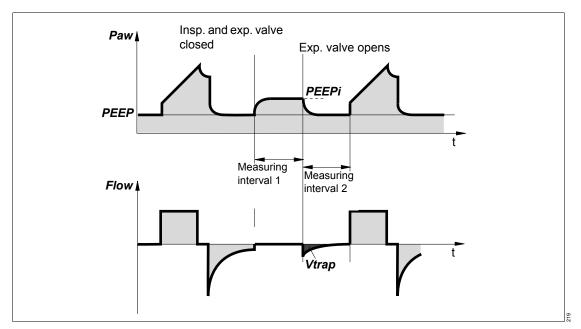
Intrinsic PEEP is the actual end-expiratory pressure inside the lungs. Owing to dynamic influences of the lung mechanics (resistance, compliance, closing volume) and the ventilation setting parameters, the Intrinsic PEEP may deviate from the PEEP in the upper airways.
