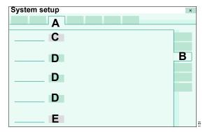
Evita V500 displays the start mode (C) and 3 ventilation modes (D). These ventilation modes are displayed in the *Ventilation settings* dialog window after Evita V500 has been started.
