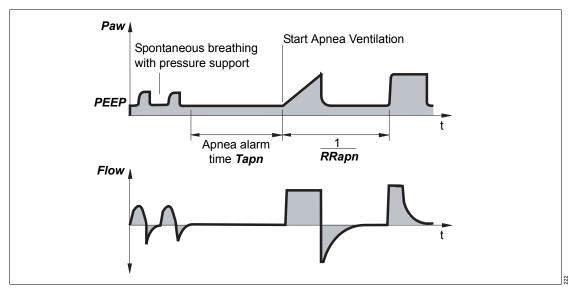
If the patient is ventilated using a volume-controlled mode without AutoFlow, apnea ventilation is also volume-controlled without AutoFlow. In all other cases, apnea ventilation is volume-controlled with AutoFlow.
