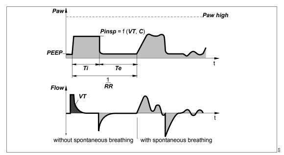
Evita V500 provides ventilation with AutoFlow/Volume Guarantee with a decreasing flow in order to avoid pressure peaks. Evita V500 determines the pressure required for the set tidal volume, with consideration of the lung conditions (compliance, resistance) and the patient's spontaneous breathing demand.
