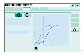
2 Touch the *Retr. Ref.* button (B) until the desired PV-Loop is displayed.
