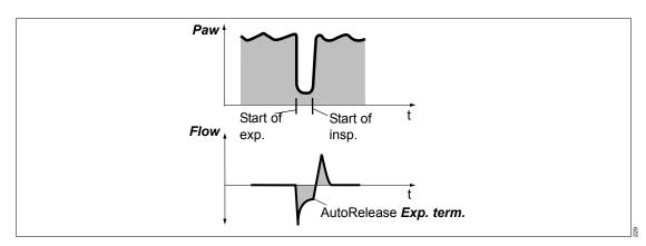
In ventilation mode PC-APRV, the duration of pressure release is determined from the expiratory flow curve when *AutoRelease* is activated. The *Exp. term.* setting specifies when the ventilation returns to the pressure level *Phigh* dependent on the decline in percent of the peak expiratory flow. The therapy control *Tlow max* limits the maximum duration of pressure release.
