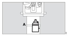
Clamp the breathing gas humidifier to the standard rail (A) under the ventilation unit and screw firmly into place.
