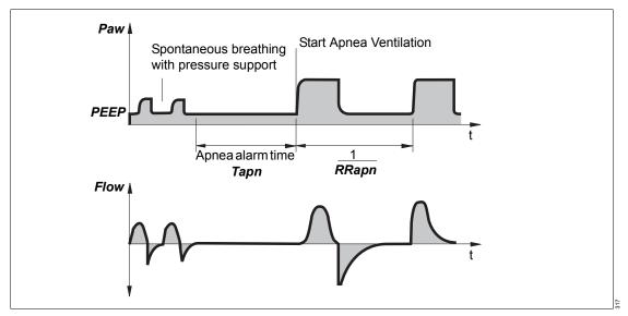
For Evita V500 to be able to detect an apnea, flow measurement with the neonatal flow sensor must function and flow monitoring with the neonatal flow sensor must be activated.
