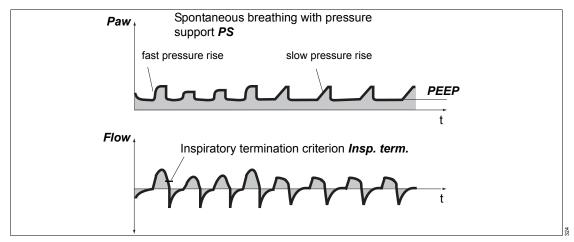
Pressure controlled ventilation is frequently used when weaning the patient from ventilation. Various additional device functions can be combined with the SPN-CPAP/PS ventilation mode. The same applies to *Variable PS*. The basic principle of pressure supported spontaneous breathing is fully retained and is not modified.
