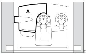
1 Open the flap (A) by lifting the lower edge upwards.
