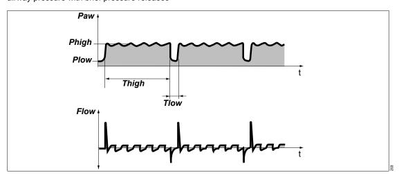
The patient breathes spontaneously at a high pressure level *Phigh* for an adjustable length of time *Thigh*. For very short expiratory times *Tlow*, Evita V500 switches to a low pressure level *Plow*. The normal lung areas are emptied, but the "slow" lung areas only change volume to a lesser extent\*.
