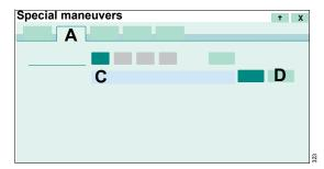
Touch the Off button (D) and confirm with the rotary knob.
