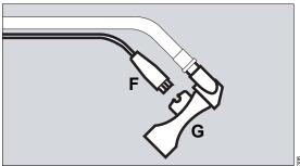
1 Disconnect plug (F) of the flow sensor cable from the neonatal flow sensor (G).
