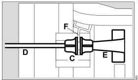
3 Clip the protective sleeve (C) immediately after the connector (E) onto the system cable (D). Align the protective sleeve so that the slots of the protective sleeve are facing downwards and upwards.
