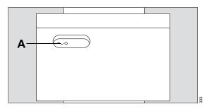
**A** LED  $\sim$  for display of mains power supply (if separate mains plug is available)
