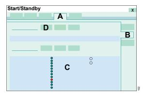
Evita V500 displays the individual test steps in a list (C). The size of the list depends on the available applications.
