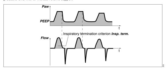
For volume support **VS**, every inspiratory effort by the patient on the PEEP level that meets the trigger criteria triggers a volume-supported breath. By setting the trigger level, the patient's inspiratory efforts are synchronized. The time, number and duration of volume-supported breaths is determined by the patient's spontaneous breathing. The pressure rise is determined by the **Slope** setting.
