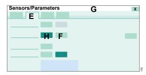
3 Touch the Off button (F) and confirm with the rotary knob.
