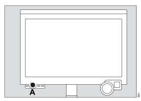
2 Press the (h) key (A) on Infinity C500. Evita V500 opens the **Shut down device** dialog.
