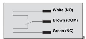
As soon as Evita V500 signals an alarm, the connection between the white cable and the brown cable (NO and COM) is closed and the nurse call is activated.
