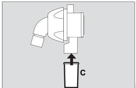
**3** Fit the collection container for the water trap (C).
