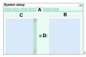
Evita V500 displays the already installed applications (B) and the applications available on the SIM card (C).
