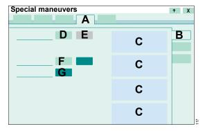
Evita V500 displays the P0.1 values of the 4 previous measurements (C).
