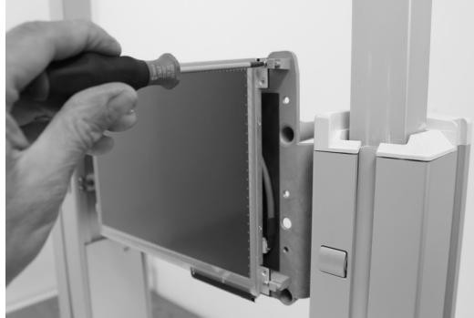
FIGURE 7-66. Remove Thread Forming Screws
