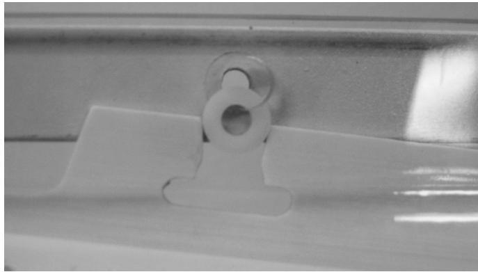
FIGURE 7-8. Using North Seal to Help Position Washers
