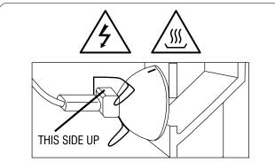
IMPORTANT: Do not touch bulb or mirror with fingers. Position bulb so that "THIS SIDE UP" faces up and the black line is centered at the top of the circular cutout in the metal housing . Be sure that the bulb seats completely in the groove in the metal housing. SEE OPERATION AND MAINTENANCE MANUAL FOR COMPLETE INSTRUCTIONS. Use only Ohmeda Medical replacement bulb part number 6600-0235-850.
