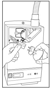
**CAUTION** (A) To avoid damage to equipment, install bulb before powering unit.
