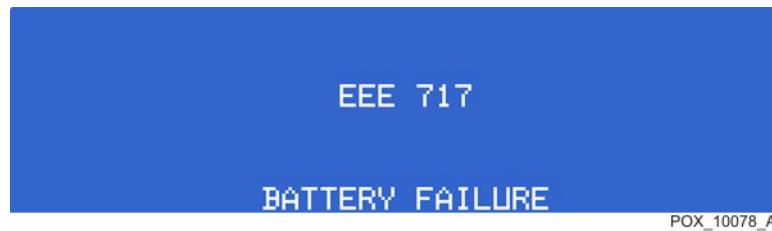
Figure 120. Error Condition Screen, Battery Failure
