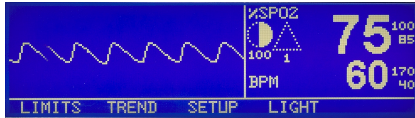
Figure 102. PLETH Display with SRC-MAX decrease in %SpO 2 of 75 with high light condition
