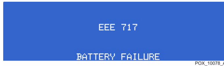
Figure 19. Error Condition Screen, Battery Failure
