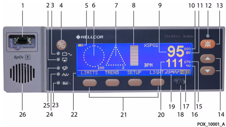
Figure 2. OxiMax N-600x Pulse Oximeter Front Panel
