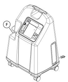
6. When placing the humidifier bottle in the compartment (F) on the concentrator, attach the humidifier bottle/adapter tube (H) to the oxygen outlet connector (1) on the concentrator.
