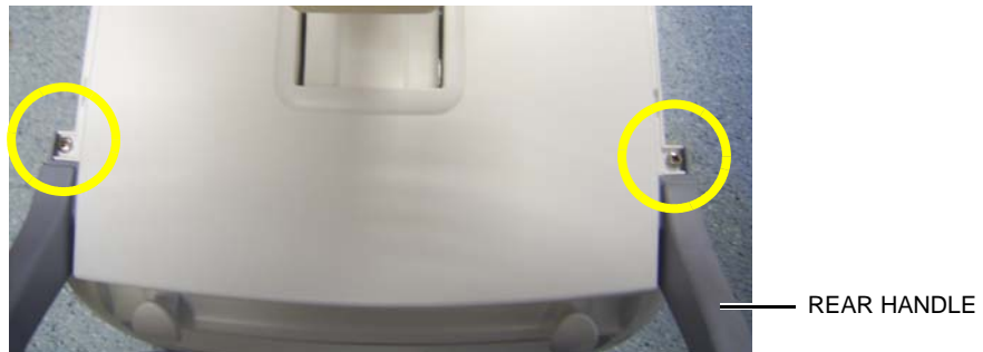
Figure 8-8 Top Cover fixing screws (seen from above)
