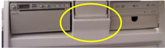
Figure 8-27 Position the column cover tab inside the front cover
