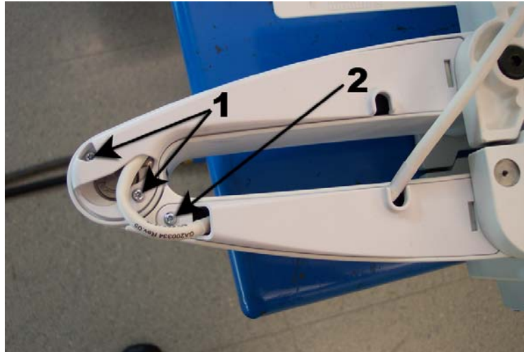
Figure 8-29 XY / Frogleg mechanism covers, right side frog leg, from underneath
