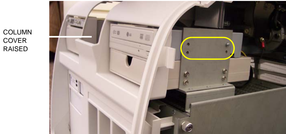
Figure 8-204 Screw placement for right side of DVD R/W drive
