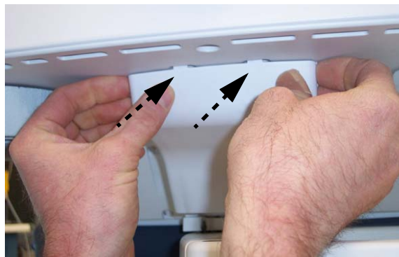
Figure 8-34 Upper tab lock placement on Bulkhead Cover
