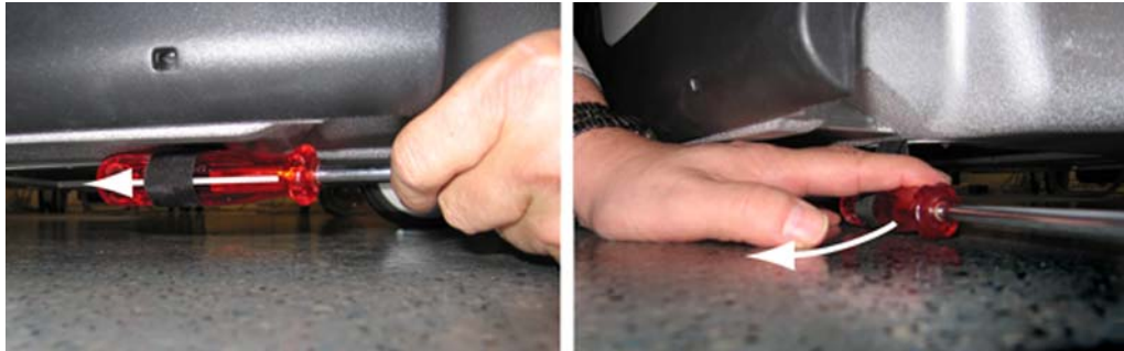
Figure 8-161 Release of the bottom air filter
