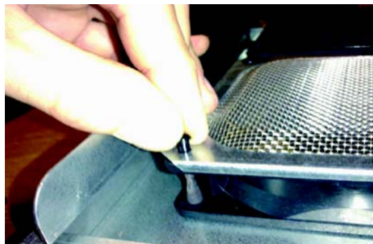
Figure 8-166 New Fan Screen and Fan Scree Frame ontop of the fan
