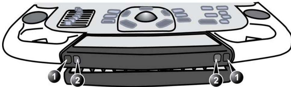
Figure 4-9 Top Console adjustment controls
