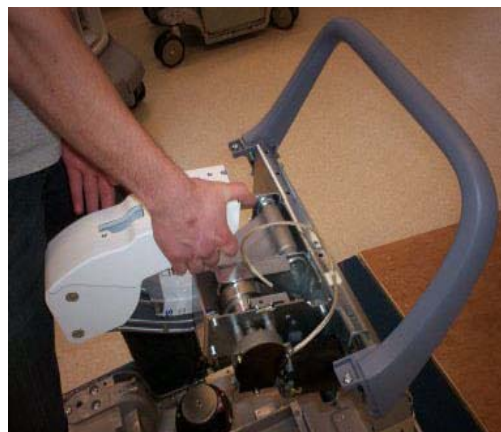
Figure 8-152 Lift the Z-Mechanism away.
