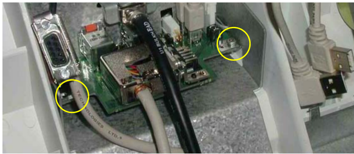
Figure 8-128 Bulkhead Board screws
