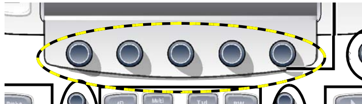
Figure 8-129 Remove five knobs
