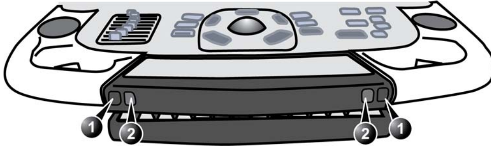
Figure 8-137 Top Console adjustment controls
