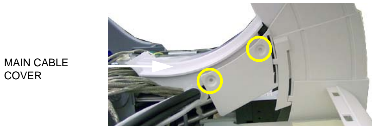
Figure 8-24 With console raised, left side screw placement
