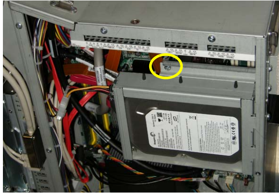
Figure 8-192 BEP Hard Disk Drive screw
