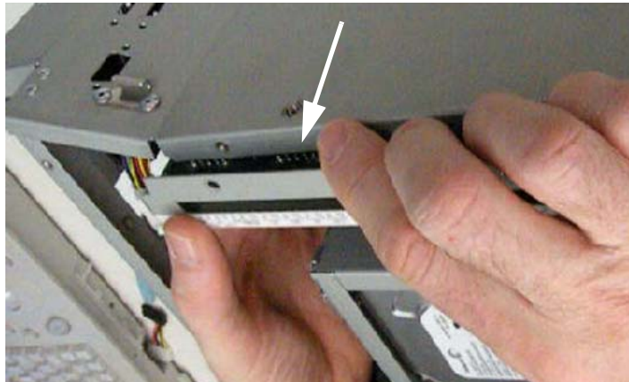
Figure 8-189 BEP Power Supply removal
