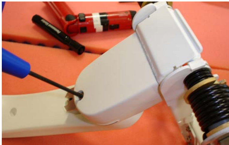
Figure 8-60 Third Arm Section Cover Removal
