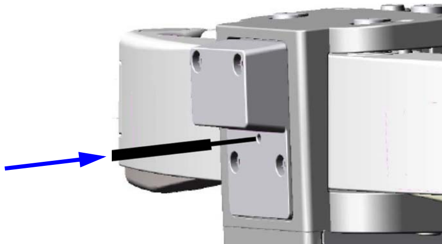
Figure 4-11 Manually releasing the XY Lock
