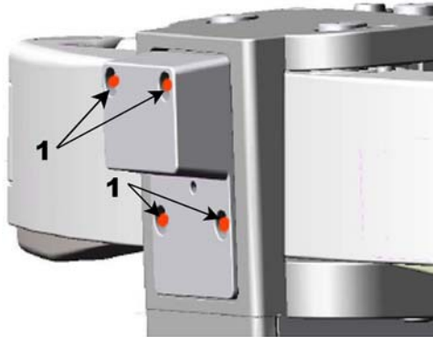
Figure 6-14 Remove the Park Lock
