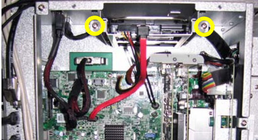
Figure 8-190 BEP6 HDD screws
