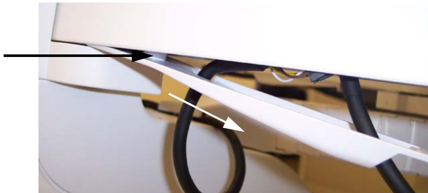
Figure 8-30 Pull down and slide XY cover out
