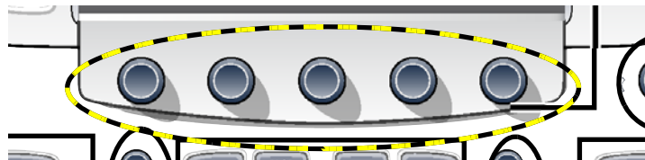
Figure 8-77 Remove five knobs
