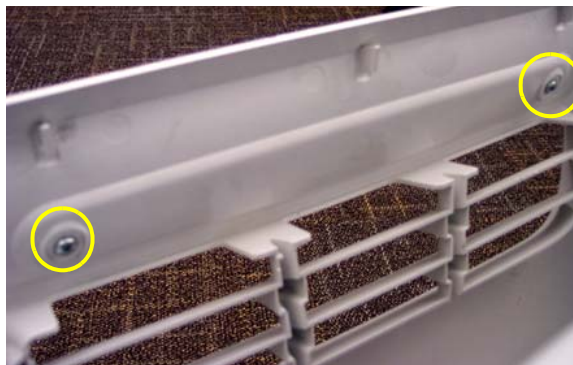
Figure 8-19 Cable Hook screw placement
