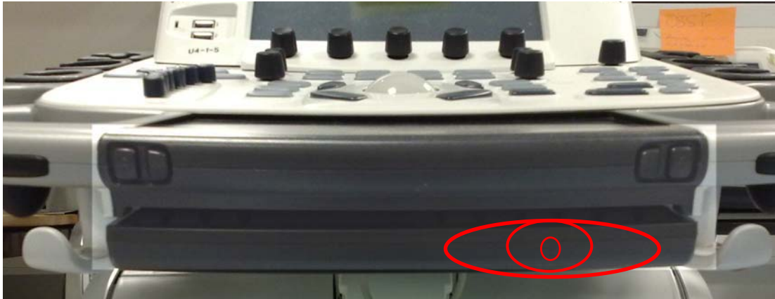
Figure 7-6 Best area to press to release (or lock) the alphanumeric keyboard
