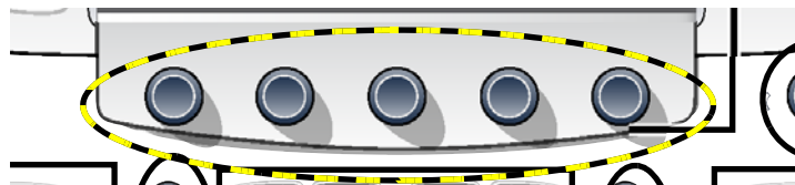
Figure 8-88 Remove five knobs
