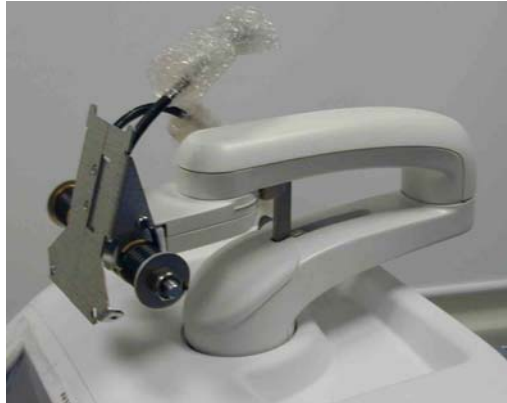
Figure 8-54 LCD Arm installed onto the UI Frame Upper (Arm for 17" screen illustrated)
