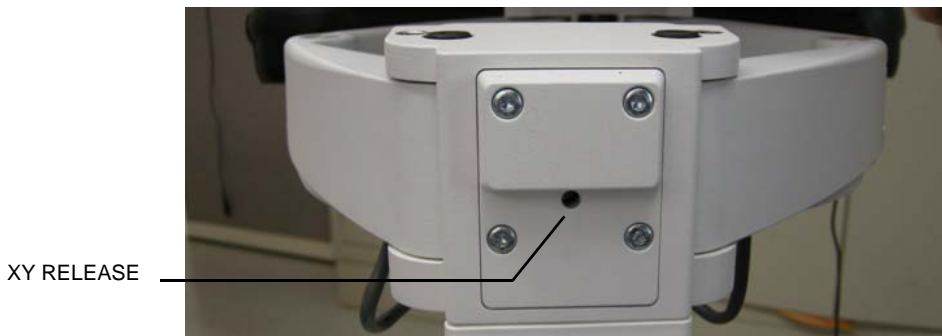
Figure 8-69 XY / Frogleg mechanism release
