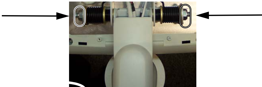
Figure 6-4 Adjusting LCD Hinge Nuts
