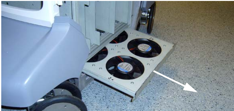
Figure 8-163 Fan Assembly removal
