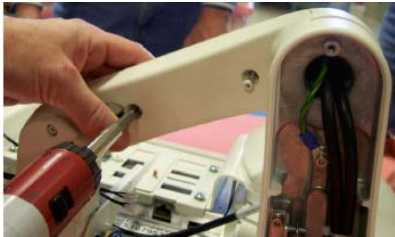
Figure 8-61 Second Arm Section Cover Removal
