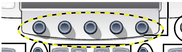
Figure 8-169 Remove five knobs
