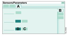
4 Touch the *Off* button (C) and confirm with the rotary knob.
