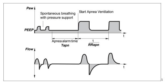
For Babylog VN500 to be able to detect an apnea, flow measurement with the neonatal flow sensor must function and flow monitoring with the neonatal flow sensor must be activated.
