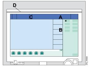
If the alarm message field (A) contains more alarms than can be displayed, the *More...* button (C) appears in the header bar. Touching this button opens the page containing all the active alarms.
