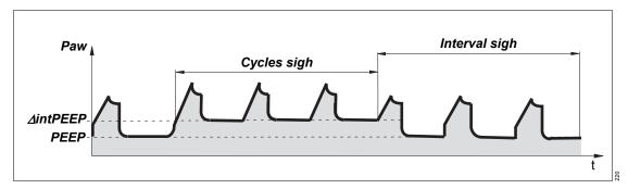
Atelectasis can be prevented by activating the sigh function and setting the sigh in the form of an intermittent PEEP. The purpose of expiratory sigh is to open collapsed areas of the lungs or to keep open "more dependent" areas of the lungs.
