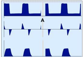
The current curves are immediately frozen. The cursor (A) displays the time of "freezing" and the value at the cursor position.
