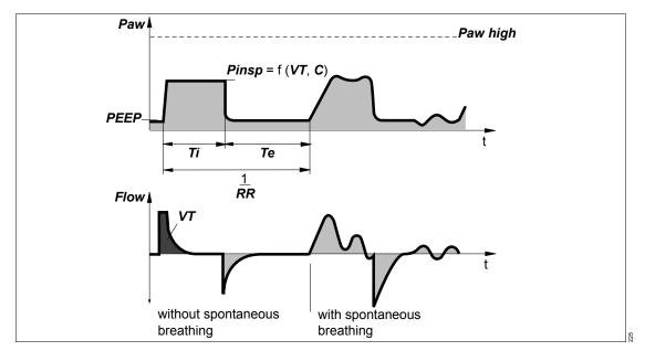
The mandatory breaths are volume controlled with the **Volume Guarantee** additional setting. To apply the set tidal volume, Babylog VN500 controls the inspiratory plateau pressure **Pinsp**.
