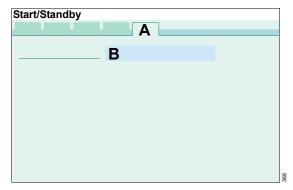
In field (B) Babylog VN500 displays the time until it is recommended to exchange the accessories.
