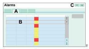
All the current alarm messages are displayed chronologically with the corresponding duration, priority and alarm message text in the list (B).
