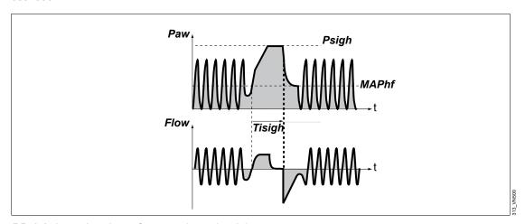
**RRsigh** determines how often per minute the sigh is to occur. A conventional pressure-controlled breath is applied with pressure **Psigh**. The duration of this breath is set with **Tisigh**. The high-frequency oscillations are discontinued for at least 150 ms prior to the sigh and are resumed 250 ms after the sigh. The high-frequency oscillations start with an expiration.
