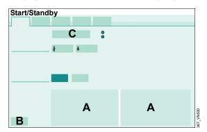
**2** Touch the **Start ventilation** button (C) and confirm with the rotary knob.
