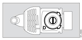
**4** Fit the diaphragm onto the edge of the fitting (D).
