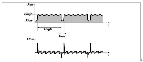
The patient breathes spontaneously at a high pressure level *Phigh* for an adjustable length of time *Thigh*. For very short expiratory times *Tlow*, Babylog VN500 switches to a low pressure level *Plow*. The normal lung areas are emptied, but the "slow" lung areas only change volume to a lesser extent\*.
