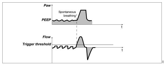
With the *Flow trigger* threshold, the mandatory breaths are synchronized with the inspiratory efforts. The start setting of the flow trigger can be configured on the *System setup* > *Ventilation* > *Start settings* > *VT, RR, Trigger* page.
