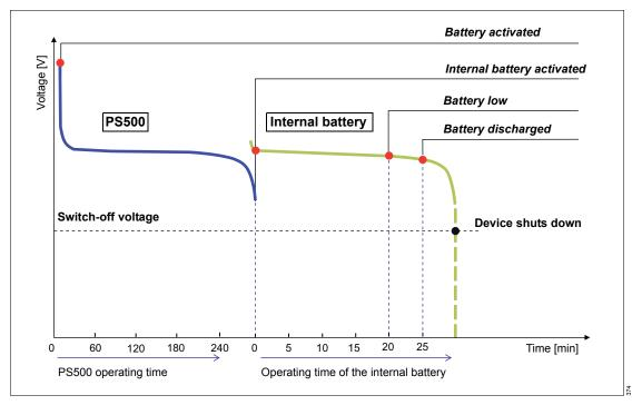
The schematic representation of the sequence of alarms with respect to battery utilization is shown in an example with a PS500 but without the use of a GS500. The representation corresponds to the operating time of new and fully charged batteries.
