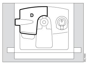
Open the flap (D) by lifting the lower edge upwards.
