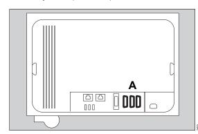
Connect an external device to the OO COM 1, COM 2 or COM 3 (A) interface of Infinity C500. Use MEDIBUS cable 8416326.
