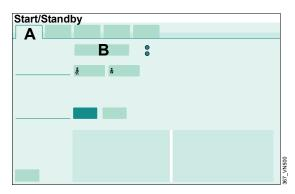
2 Touch the *Standby* button (B) and confirm with the rotary knob.
