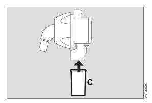
**3** Fit the water trap container (C).
