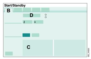
Babylog VN500 displays the ventilation parameter start-up settings. The **Start ventilation** button (D) can be used to start the therapy. When the therapy is started, the settings become effective.
