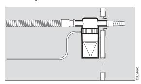
Push the inlet port or the outlet port of the medication nebulizer into the upper hose guide of the incubator.
