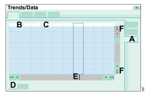
The trend values for the parameters (B) with the units are displayed in 7 to 8 time columns (C). Use the buttons (F) to scroll in the trend table.
