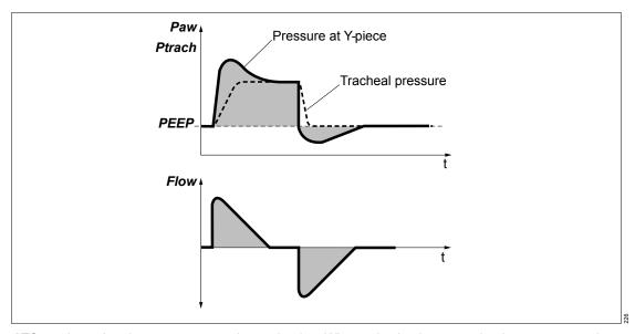
**ATC** regulates the airway pressure to the tracheal level. This function calculates and displays the tracheal pressure on the basis of a mathematical tube model, the set tube type and the inner diameter of the tube.
