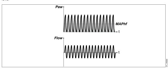
Ventilation with high-frequency pressure oscillations enables gas to be exchanged in the lungs despite very small tidal volumes (often in the
