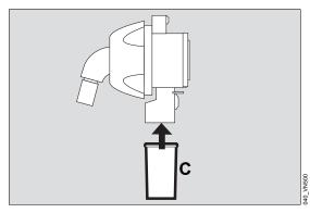
4 Fit the water trap container (C).
