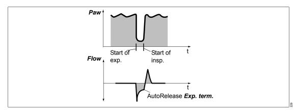
In ventilation mode PC-APRV, the duration of pressure release is determined from the expiratory flow curve when *AutoRelease* is activated. The *Exp. term.* setting specifies when the ventilation returns to the pressure level *Phigh* dependent on the decline in percent of the peak expiratory flow. The therapy control *Phigh* limits the maximum duration of pressure release.
