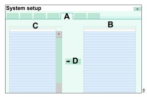
Babylog VN500 displays the already installed applications (B) and the applications available on the SIM card (C).
