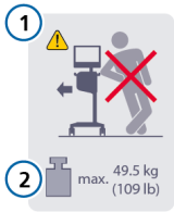
Figure 16-5. Trolley warning stickers
