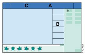
If the alarm message field contains more alarms than can be displayed, the *More...* button (C) appears in the header bar. Touching this button opens the page containing all the active alarms.
