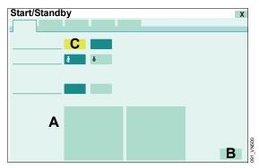
2 Touch the *Start* button (C) and confirm with the rotary knob.
