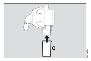
Fit the collection container for the water trap (C).
