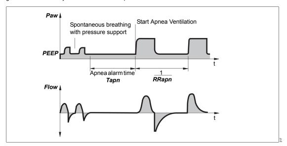
For Babylog VN500 to be able to detect an apnea, flow measurement with the neonatal flow sensor must function and flow monitoring with the neonatal flow sensor must be activated.
