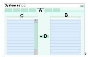
Babylog VN500 displays the already installed applications (B) and the applications available on the SIM card (C).
