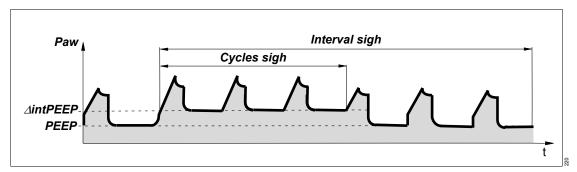
Atelectasis can be prevented by activating the sigh function and setting the sigh in the form of an intermittent PEEP. The purpose of expiratory sigh is to open collapsed areas of the lung or to keep open "more dependent" areas of the lung.
