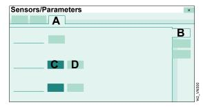
3 Touch the Reusable (C) or Disposable (D) button and confirm with the rotary knob.
