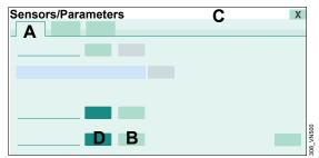
3 Touch the Off button (B) and confirm with the rotary knob. Babylog VN500 displays the following information in the message field (C): *External monitoring must be used!*
