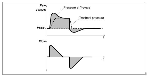
**ATC** controls the airway pressure at the tracheal level. This function calculates and displays the tracheal pressure on the basis of a mathematical tube model, the set tube type and the inner diameter of the tube.
