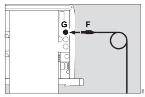
5 Insert the connector (F) of the flow sensor cable into the socket (G) at the rear of Babylog VN500.
