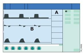
The parameters can be displayed in parameter fields (A) and in the curve field (B).
