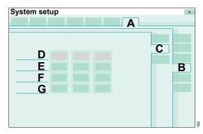
The settings for **COM 1**, **COM 2**, and **COM 3** are displayed. **MEDIBUS** or **MEDIBUS.X** can be selected for the **Protocol** parameter.
