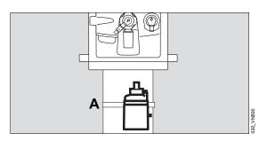
Clamp the breathing gas humidifier to the standard rail (A) under the ventilation unit and screw firmly into place.
