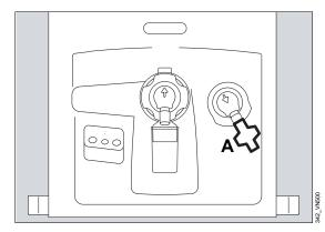
Fit the bacterial filter (A) onto the inspiratory port.
