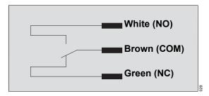
As soon as Babylog VN500 signals an alarm, the connection between the white cable and the brown cable (NO and COM) is closed and the nurse call is activated.
