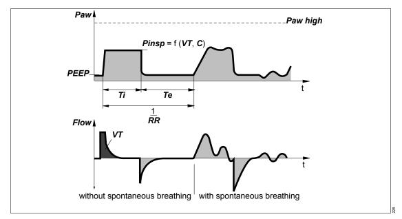
With the **Volume Guarantee** additional setting, the mandatory breaths are volume controlled. To apply the set tidal volume, Babylog VN500 controls the inspiratory plateau pressure **Pinsp**.
