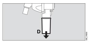
3 Remove the collection container (D) from the water trap. Empty the collection container. Observe the hospital hygiene regulations!
