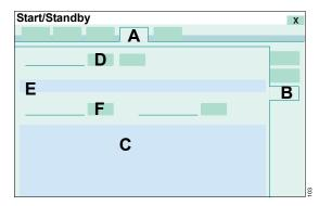
The values of the last test are displayed (C). If a valid measurement has not yet taken place, the standard values are displayed.
