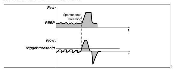
With the *Flow trigger* threshold, the mandatory breaths are synchronized with the inspiratory efforts. The start setting of the flow trigger can be configured on the page *System setup > Ventilation > Start settings > VT, RR, Trigger*.
