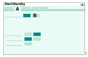
4 Touch the *NIV* button (B) and confirm with the rotary knob.
