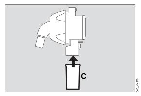
**4** Fit the collection container for the water trap (C).
