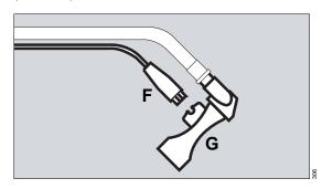
1 Disconnect plug (F) of the flow sensor cable from the neonatal flow sensor (G).
