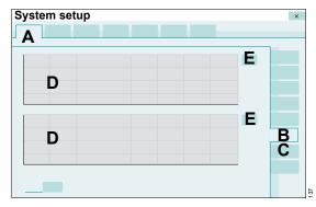
Each page contains 2 graphic trend displays (D). A maximum of 3 parameters can be configured for each trend display.
