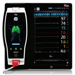
The Handheld snaps into Root. Root charges the Handheld and displays Handheld parameters.
