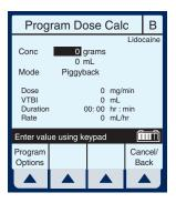
To override the Piggyback Delivery Mode default, scroll down to Mode using ▼, then select ▲ [CHANGE MODE].
