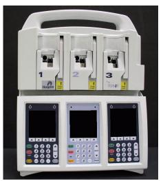
The Plum A+ and Plum A+3 Volumetric Infusion Systems are designed to meet the fluid delivery requirements of today's evolving healthcare environments. Both are cassette based multifunction infusion systems. The Plum A+ allows two lines in and one line out while the Plum A+3 allows six lines in and three lines out. Each pump can be used for standard, piggyback, or concurrent delivery. Therapy modes include:
