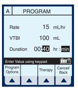
**NOTE:** When DURATION is changed, RATE is automatically
