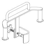
Always mount the tandem carrier (List# 12270-01) to the pole before attaching the infuser(s) to the tandem carrier.
