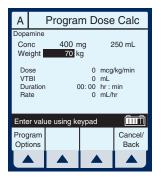
**NOTE:** The Concentration elements and weight value must be entered before the [SELECT] keys allow access to remaining fields.
