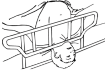
Entrapment under the bed rail
