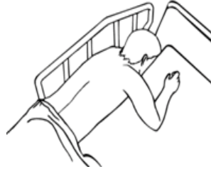
Entrapment between the bed rail and mattress
