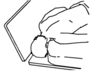
Entrapment between the end of the rail and the side edge of the headboard or foot board
