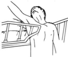
Entrapment between split bed rails
