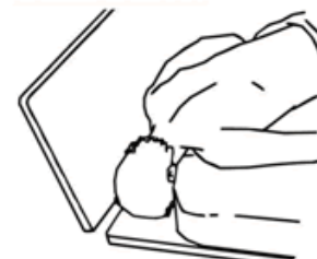
Entrapment between the end of the rail and the side edge of the headboard or foot board
