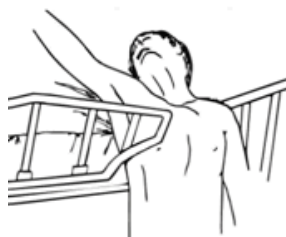
Entrapment between split bed rails
