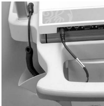
Correct amount of cable slack.
