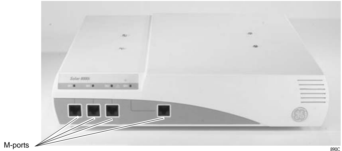
Front View of the Processing Unit
