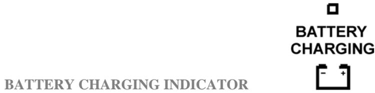
The yellow CHARGING LED illuminates when the monitor's batteries are charging. The CHARGING LED will not be illuminated when the batteries are fully charged, or when the monitor is not connected to AC power.
