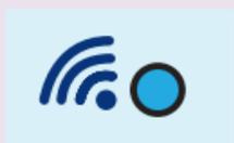
The Communicating indicator (blue) is on whenever the pump is communicating with the PharmGuard® Server using wireless or wired interface. There is no audible tone associate with communications. During normal network operations the light may periodically turn on and off. The Communicating indicator has no affect on clinical operations of the pump.
