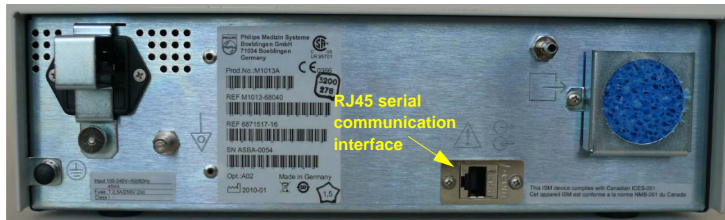
Figure 6 RJ45 connection on the back of the gas analyzer
