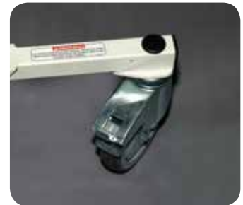
c. Lock caster (shown in locked position)
