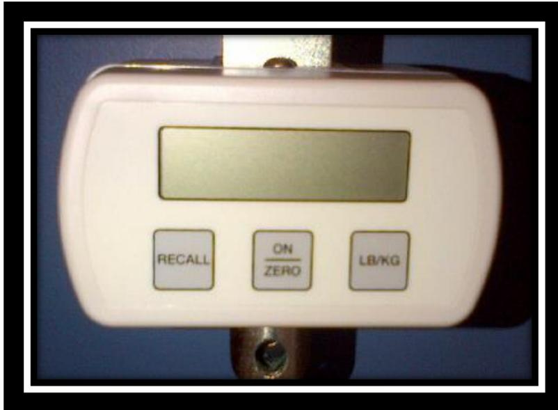
1. Fit the sling to the spreader bar and then press the **ON/ZERO** button to start or zero the scale.
