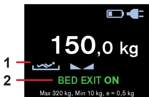
Fig. Display description (Bed Exit Alarm Monitoring)
